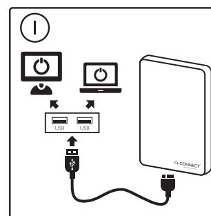
1. Turn on your computer and connect the external HDD to a USB 3.0 port of your computer, by using the USB 3.0 data cable provided.
